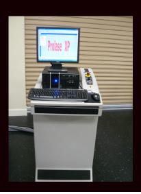
TJS, Inc has designed and developed a Windows interface for the Control Laser Corporation Insignia LX900 and Icon LS900 lasers.
